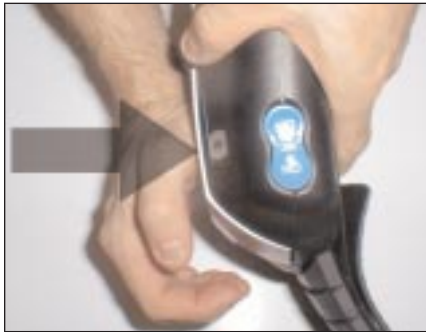
Figure 10: Filter Cover Removal, Step 1 Place the Turbo Unit upright on a stable surface, such as a table. With the heel of your right palm, push firmly on the second column of air holes of the silver Filter Cover; the Cover will deflect slightly.
