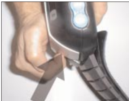
Figure 11: Filter Cover Removal, Step 2 While continuing to slightly deflect the silver Filter Cover, press your fingers down on groove of the black latch until it releases.
