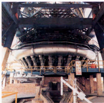
Tuyere stock expansion joints for a blast furnace. Iron and steel industry applications also include hot and cold blast mains, gas mains and fume extraction systems.
