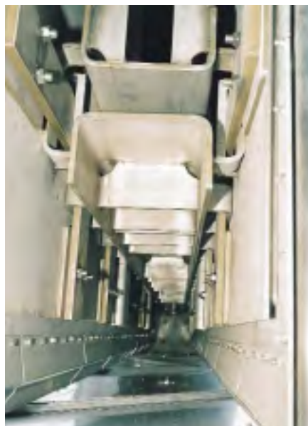
"Sandwich" blade construction. One single blade consists of seven independent modules, all designed to accommodate sharply rising and falling gas temperatures.
