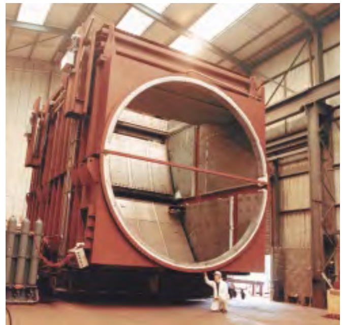
Three blade diverter damper for power station in China.
