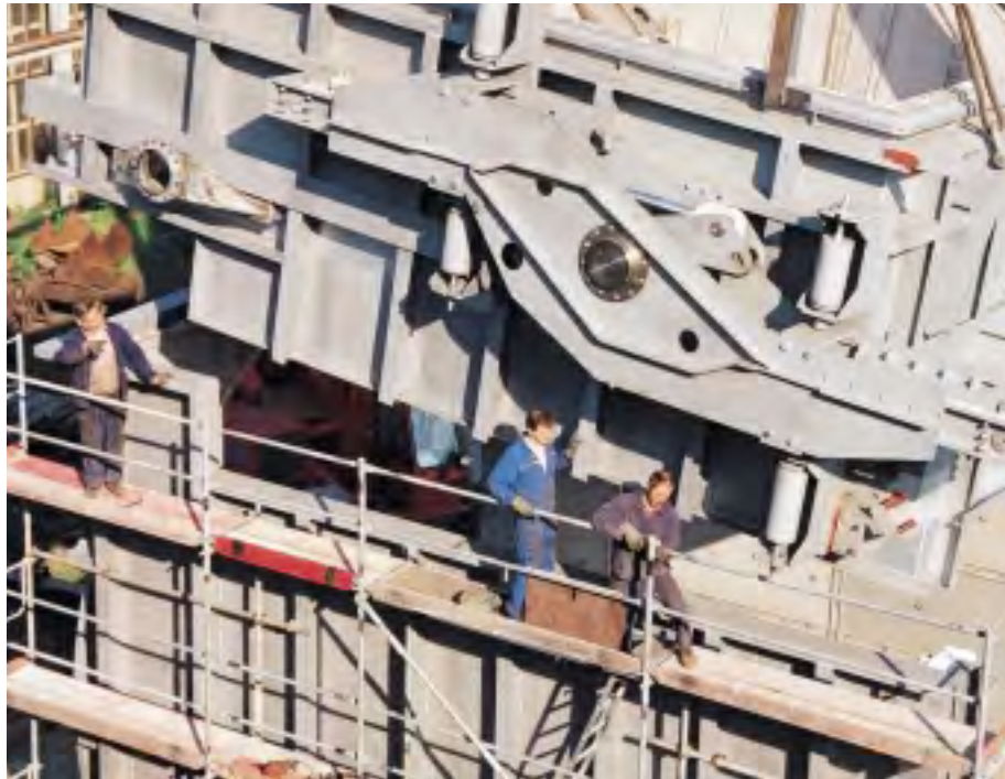
Test assembly of a hydraulically-operated diverter for a V94.3A turbine.
