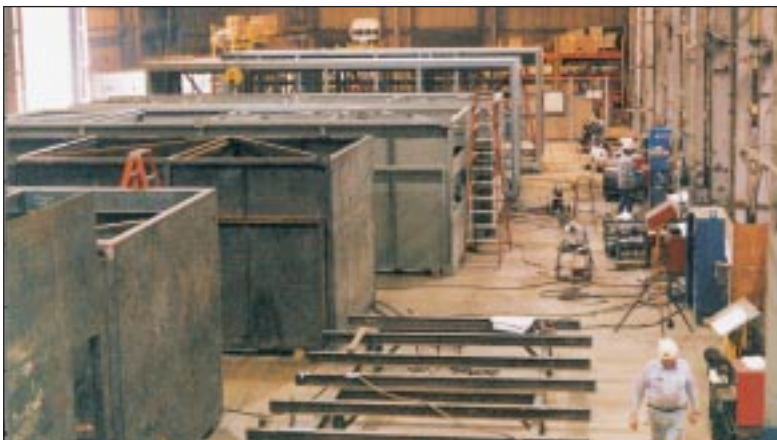
GE Frame 7FA filterhouse modules in production.
