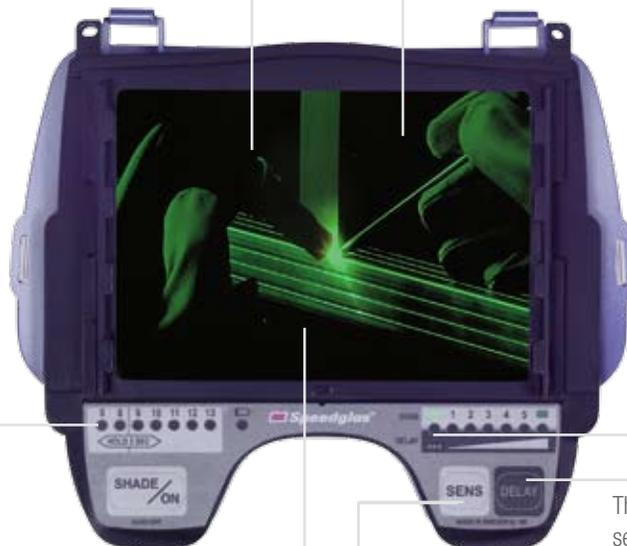
The 'tack welding comfort mode' uses an intermediate light state (shade 5). If a follow-up arc is not struck within two seconds, the welding filter switches to the normal light state (shade 3). The comfort mode may help reduce eye fatigue resulting from the eye constantly needing to adjust to differing light levels during tack welding.
